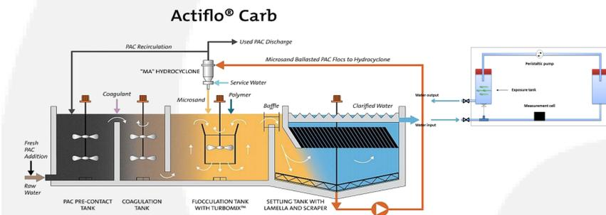
Figure 1. Scheme of the Actiflo® Carb technology to remove micropollutants.
