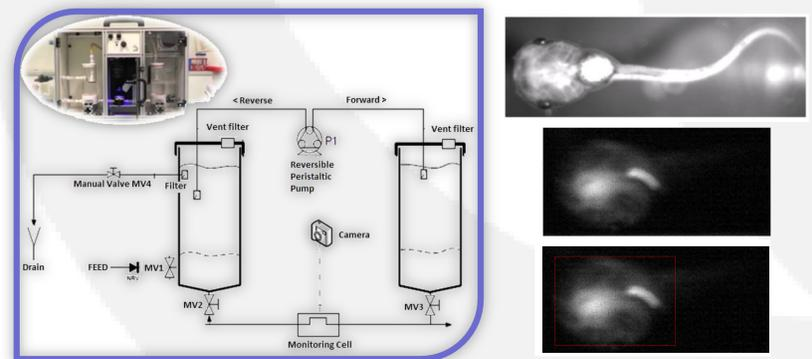
Figure 2. Scheme of the on-line readout system (left) to the endocrine disruption assessment. (Top right) Photo of tadpole in white light, offline. (Middle right) Image of the fluorescent part in blue light, acquired with the on-line readout system of figure 3. (Bottom right) Detection of the fluorescent part with image processing algorithms.
